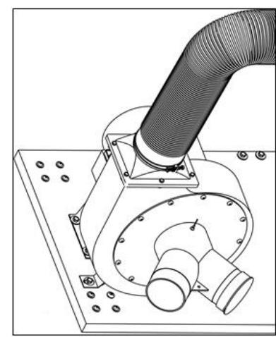
10. The dust collector is now ready to be used. The dust collector can be connected to the machine it was meant for, make sure to use a proper connecting hose and that it is firmly connected to both the inlet of the dust collector as the connector on the machine.
