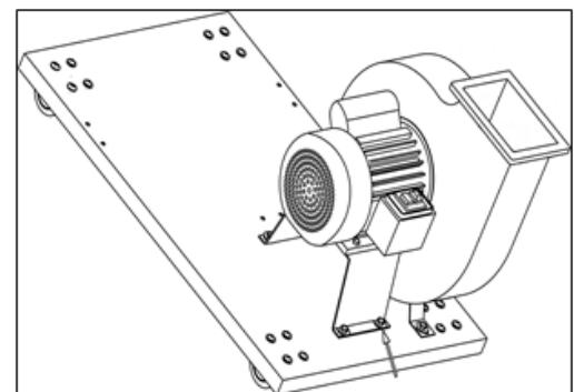
3. Mount the outlet (L) to the fan, first place the seal (I) and then the outlet. Mount it with the bolts, rings and nuts.
