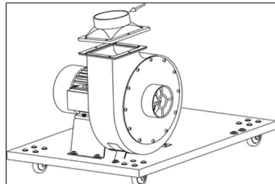
4. Mount the lower supports on the carriage with the bolts, rings and nuts.
