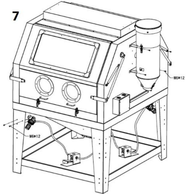
8. Place the dust extractor against the cabinet and mount it with the M6x12mm bolts and M6 nuts, use calking/kit to seal the gap between the dust extractor and hole in the cabinet to prevent dust from escaping during use.
