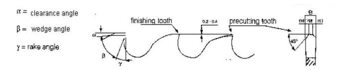
Clearance angle ß and rake angle y of the tooth have been selected correctly in view of the material to be sawn. the principle is as follows.
