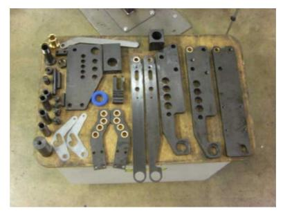
4.5 Before the major components can be assembled, you must pre-assemble some components. Looking at dwg #M050-EV2.Locate parts #2.3.7.8.9.10.11 & 20. Install bumper pins and snap rings into the plates orienting them as shown below. Note: # 7 & 8 are different lengths
