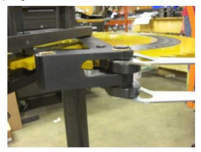
4.30 Next the anti spring back lever can be pre assembled, using dwa #M050-EV-4 locate the anti spring back lever (#7). pivot block (#8). 1/2-13x1 - 3/4 hex bolt. 1/2" lock. (2) 1/2" washers and (2) 5/16x1 hex bolts
