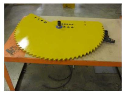
4.13 Install the latch drive bar (lower) #11 orienting as shown
