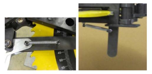
4.34 The remaining pins can be installed in their respective locations.
