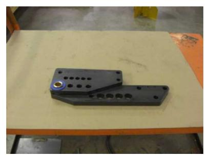
4.23 Locate the plate spacer (#4) and the rectangular spacer (#11) and fasten them to the ratchet wheel using  $5/8-11 \times 1-1/2$  with lock washers, as shown below. Do not tighten yet
