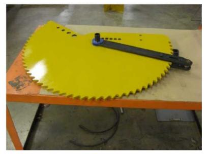
4.15 Locate the bottom plate #3 and slide onto the threaded sleeve as shown below. Make sure the short bumper pin is installed in the bottom plate as shown
