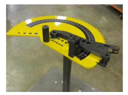
4.24 Locate the 3 long spacers (#3). short spacer (2)  $3/4-10 \ge 6.5$  HHCS. and (1)  $3/4-10 \ge 9.0$  HHCS with lock washers. Install the top plate assembly spacers and bolts as shown below. Do not tighten any of the main bolts yet.
