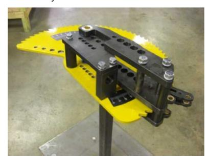
4.25 Now that the majority of the machine is built, the drive lever section can now be assembled, use dwa #M050-EV3. Locate the 2 drive links (#2) the shaft block (#4). Bolt together using (8)5/16-18 X 1" as shown below.
