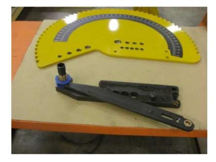
4.11 Next install the ratchet wheel # 1 onto the lower pivot sleeve.Note the orientation of the ratchet wheel because it can be put on backwards. Orient as shown below.
