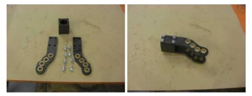
4.26 Set this assembly aside and continue with the latch drive bars from the last step. Locate spacer (#6) and bolt the drive bars together with the  $3/8-16 \times 1 - 3/4$ " flat head screw
