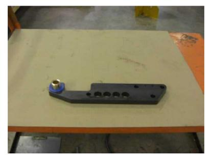
4.21 Install the hook drive Plate. This must be oriented correctly as it can be put on backwards, see picture below
