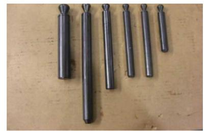
4.35 Now that the majority of the machine is assembled slide the main die pin through the center axis of the machine as well as all of the other pins. Now the 3 main bolts can be torgued to 100ft lbs. next
