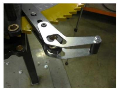
4.29 Install pivot pin (#12) through drive link, lock tab slots. upper drive bar. the drive link again. lower drive bar. and finally the lower lock tab.
