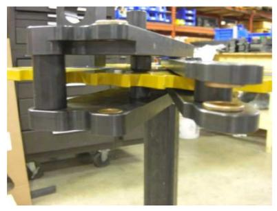
4.27 Install snap ring onto shaft (#11) and slip through drive link end hole through middle and bottom plates. and install lower snag ring to shaft (#11) as shown below
