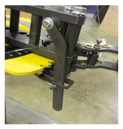
4.32 Install the lower latch plate as shown using (2) 1/4-20x3/4"
