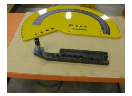
4.8 Locate the latch drive bars (upper #9 and lower #11) making sure the bumper pins are installed along with the snap rings.
