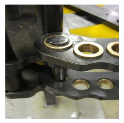
4.28 Locate lock tabs (#7). Spacer (#8). 5/8" drive pin (#5). install a 5/8" snap ring onto shaft (#5). slip shaft through holes in lock tab. upper drive lever slots and then lower drive lever slots and finally the latch plate. Install the 5/8" lower snap ring onto shaft
