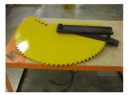
4.17 Using two people grab the partially assembled ratchet wheel assembly and flip it over lowering it onto the stand. Install the (4)  $3/8-16 \times 1$ " bolts and lock washers. Your assembly should look like the picture below.
