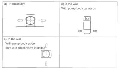
It is recommended to install a check valve in order to resume the system operation quickly and easily even after the first priming
